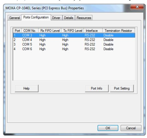
3. Select a COM number for the port from the Port Number pull-down list. Select the Auto Enumerating COM Number option to map subsequent ports automatically. The port numbers will be assigned in sequence. For example, if COM 3 is assigned to Port 1, then COM 4 (if not already occupied) will be assigned to Port 2, etc.
