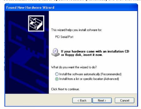
4. Select Search for the best driver in these locations, select Include this location in the search, and then click Browse. If the system is a 32-bit (x86) platform, navigate to the \CP-118EL Series\Software\Windows XP\_2003\x86 folder on the CD. If the system is a 64-bit (x64) platform, navigate to the \CP-118EL Series\Software\Windows XP\_2003\x64 folder on the CD and then click Next to continue.
