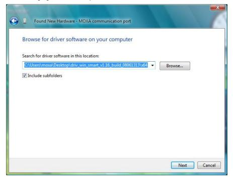
5. Wait while the installation wizard searches for the correct drivers. The next window that opens cautions you that although this software has not passed Windows Logo testing, the driver has been tested and shown that it can support the Windows OS. Click **Install this driver software anyway** to proceed.
