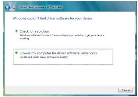
4. Select Search for driver software in this location, select Include subfolders, and then click Browse. If the system is a 32-bit (x86) platform, navigate to the \CP-114EL Series\Software\Windows 2008\_Vista\x86 folder on the CD. If the system is a 64-bit (x64) platform, navigate to the \CP-114EL Series\Software\Windows 2008\_Vista\x64 folder on the CD and then click Next to continue.
