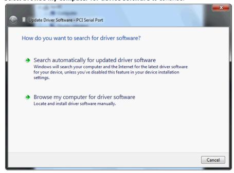
4. Select Search for driver software in this location, select Include subfolders, and then click Browse. If the system is a 32-bit (x86) platform, navigate to the \CP-104EL-A Series\Software\Windows 7\x86 folder on the CD. If the system is a 64-bit (x64) platform, navigate to the \CP-104EL-A Series\Software\Windows 7\x64 folder on the CD and then click Next to continue.
