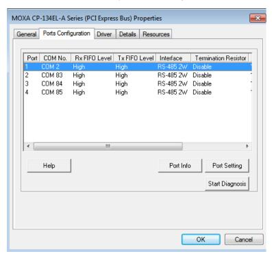
Check the Auto Enumerating COM Number option to map subsequent ports automatically. The port numbers will be assigned in sequence. Select Interface (RS-232, RS-422, RS-485-2W, or RS-485-4W) from the drop-down box. An Auto Tuning function is provided with RS-485-2W. Click OK to save the settings.
