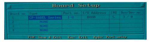
4. You may enter or modify the settings of each port at this stage. The values displayed first are the port's initial values that were set up when the driver was installed.
